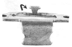
The gearshift stop plate is also notched and half gone in a critical load area. When these little guys finally give it up, your whole box could bite it. The stuff reputations are made of!
