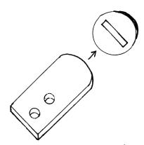
Use a piece of steel to remove the large screw plugs in the side cases without chewing them to pieces. Insert a screwdriver into a hole and use it as a lever or use a Crescent wrench to grip it. It can easily be made from scrap steel of the correct thickness by using a hacksaw, file, and drill.
